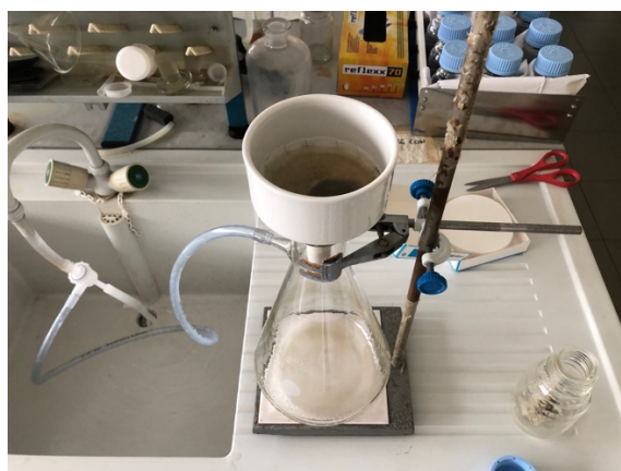
Figure 38: Vacuum filter system for the extraction of the solution obtained by shaking the plastic strips.
