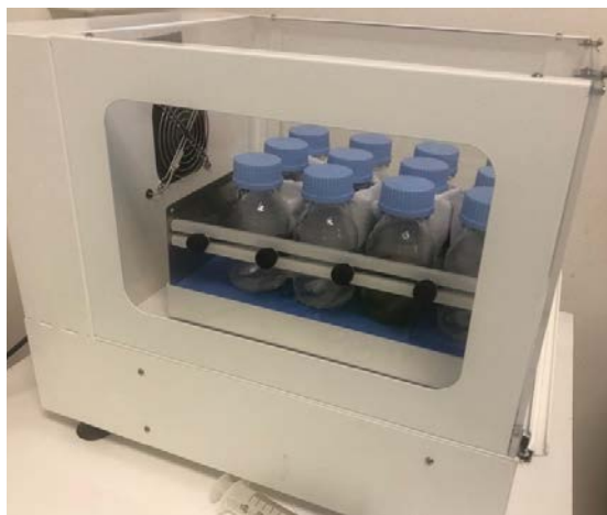
Figure 37: Glass bottles with sections of the plastic strips in agitation for performing leaching tests.
