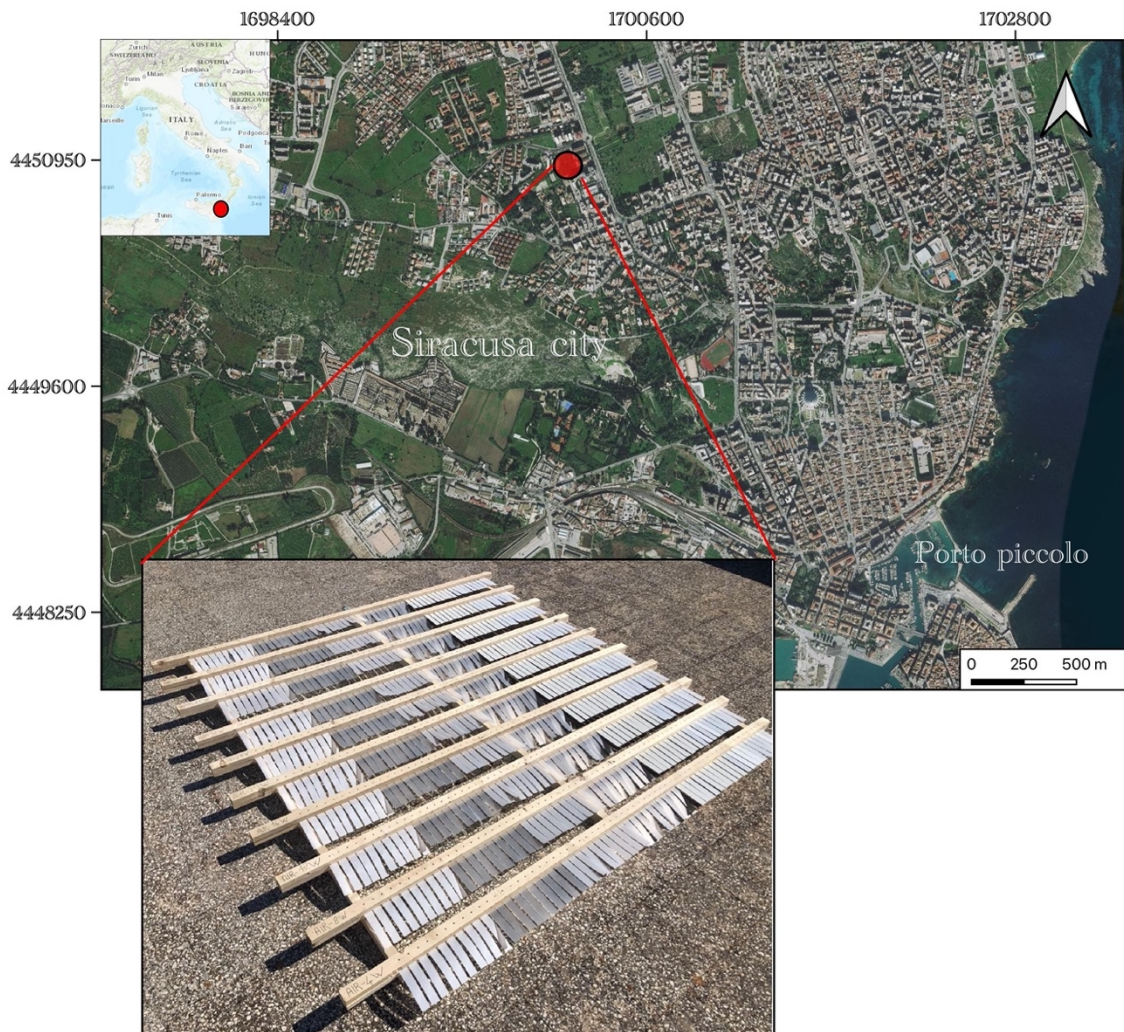
Figure 26: Testing rack installed on a terrace of a building in Siracusa.
