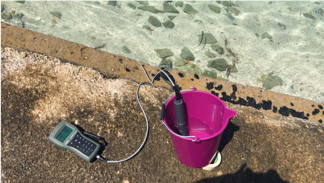
Figure 33: Measurement of chemical-physical parameters with portable logging multiparameter meter equipped with a multi-sensor probe.
