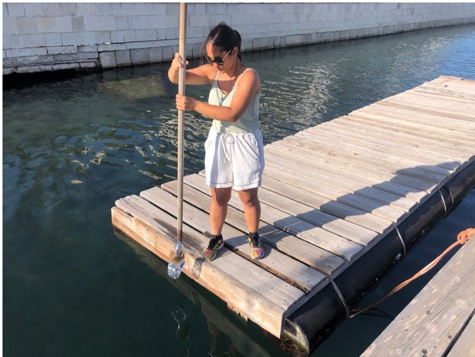
Figure 32: Rudimentary sampler by means of which water samples were taken from the bottom of the port.
