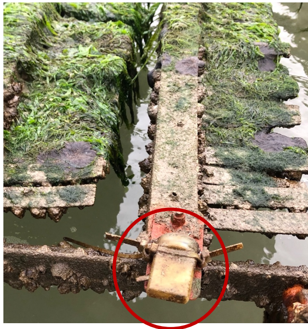
Figure 34: HOBO sensor in the intertidal lagoon environment. The light intensity data in the lagoon environment were not reliable as the strong and sudden colonization of the sensors by the biofouling, associated with logistical difficulties in cleaning the HOBO sensors, did not allow the recording in an optimal and continuous way.
