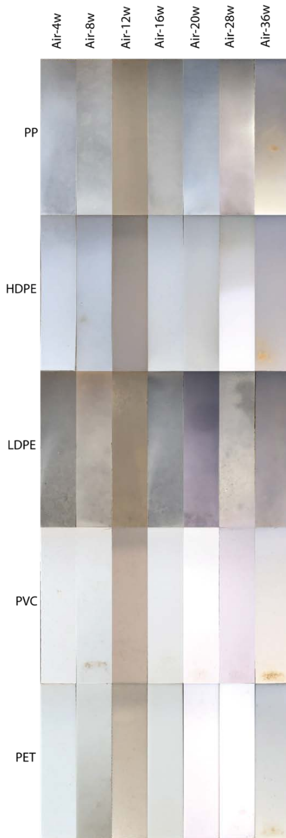
Figure 52: Temporal evolution of the different types of plastics exposed to airborne environment.
