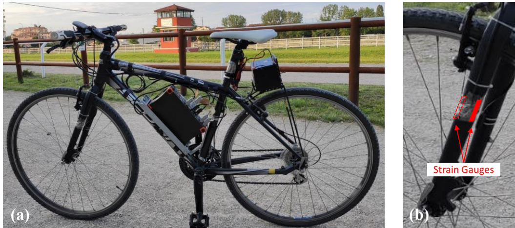
Figure 7.7. Mountain-bike: (a) overall view of the bicycle and components; (b) two strain gauges applied to the front fork.
