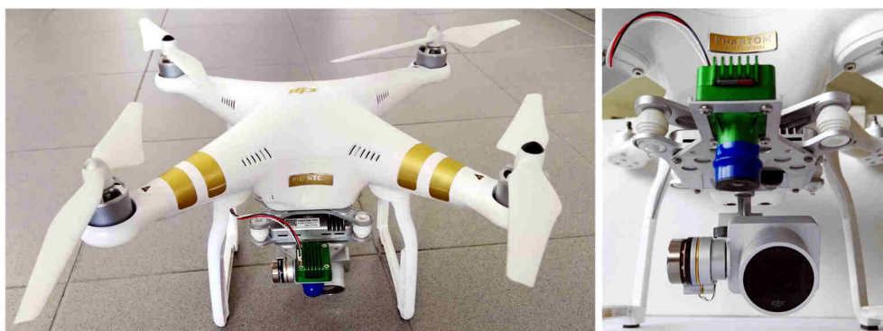
Figure 3.4 On the left: DJI Phantom 3 Professional equipped with the Sentera Single sensor. On the right: detail on both the RGB native camera of the DJI Phantom 3 and the added Sentera Single sensor, mounted in a fixed nadiral arrangement.
