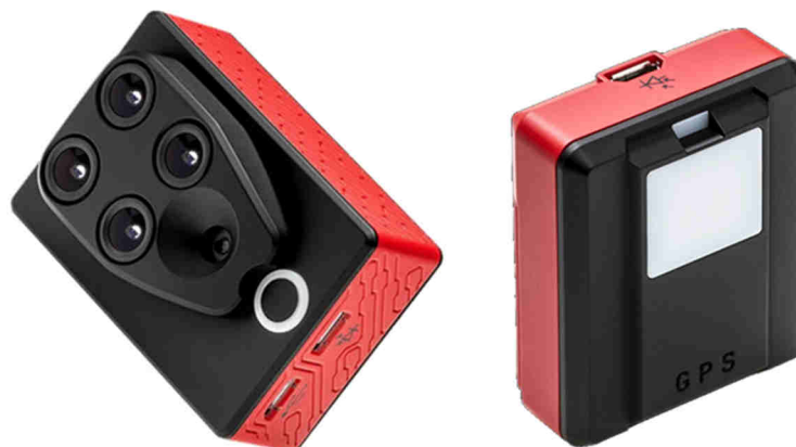
Figure 3.6 On the left: the body of the Parrot Sequoia camera. The green, red, red edge and near infrared dedicated sensors are well visible. The other optic is the 16Mpix RGB sensor. On the right: view of the top part of the downwelling light sensor (the so-called “sunshine sensor”). Beneath the “white” plastic cover there are sensors with the same characteristics of the body camera ones and equipped with the same bandpass filters, in order to measure the diffuse irradiance.
