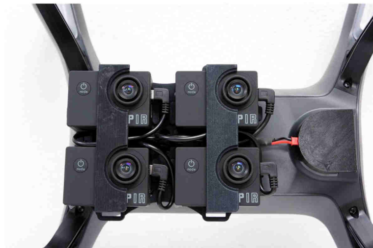
Figure 3.9 MAPIR camera mounted on a 3DR Solo with a quad static mount (source: https://www.mapir.camera/ ).
