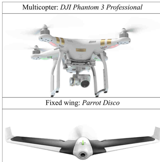
Figure 2.1 Examples of a multicopter (source: https://www.dji.com/phantom-3-pro ) and a fixed wing drone (source: https://www.parrot.com/global/drones/parrot-disco#parrot-disco ) of two of the major manufacturers.
