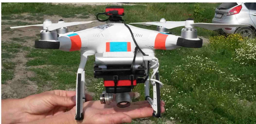
Figure 3.7 DJI Phantom 3 Professional equipped with the Parrot Sequoia: the camera (body) is mounted in a fixed nadiral arrangement, while the downwelling light sensor, containing also the GPS antenna, is on the top.
