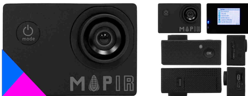
Figure 3.1 MAPIR camera “NDVI”. The dimensions are comparable to a GoPro camera. (source: https://www.mapir.camera/ accessed on August 20th, 2018).
