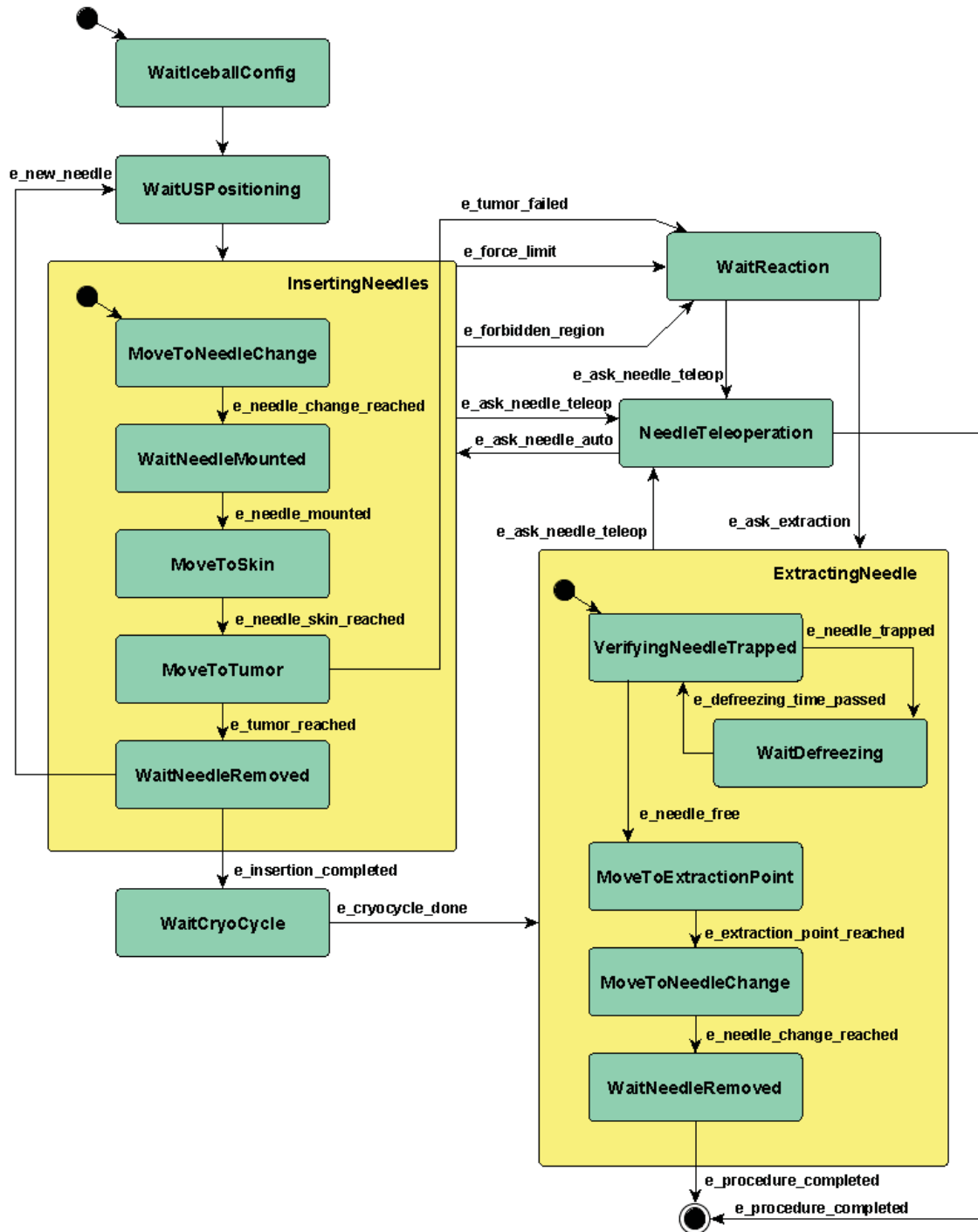
Fig. 4.8 Finite state machine for the needle insertion.
